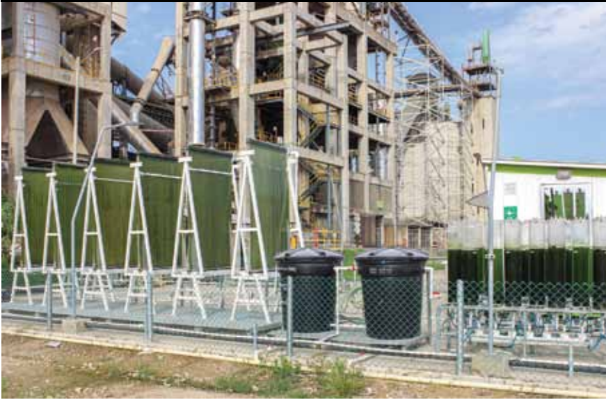
Figure 3: flat panel PBR developed by CarbonBioCapture and tested under real operating conditions at Argos' cement plant in Cartagena, Colombia, using Argos' developed process and growing medium. Tubular PBRs are used for inoculation
